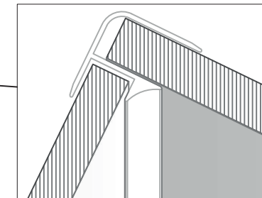
External angle profile 32x32 mm detail
